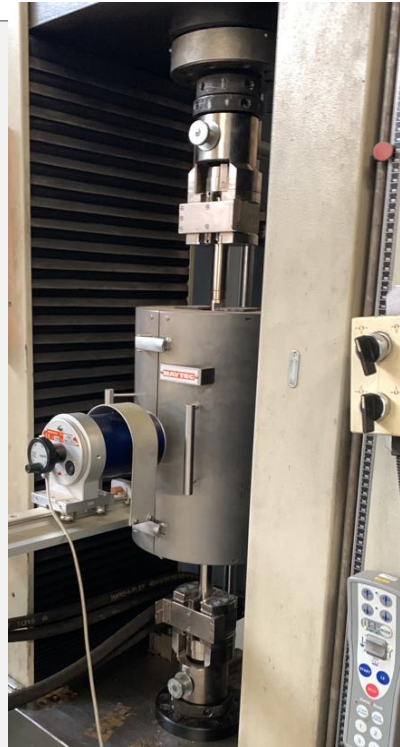
Extensometer – MAYTEC PMA-12/V7-1, HT-Extensometer up to 1500 °C
