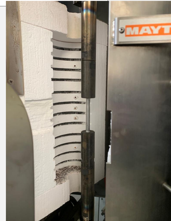
Furnace – MAYTEC HTO-08/01, Round Furnace up to 1000 °C
