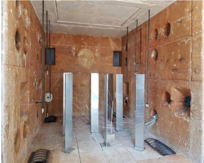
Test specimens before the fire test
